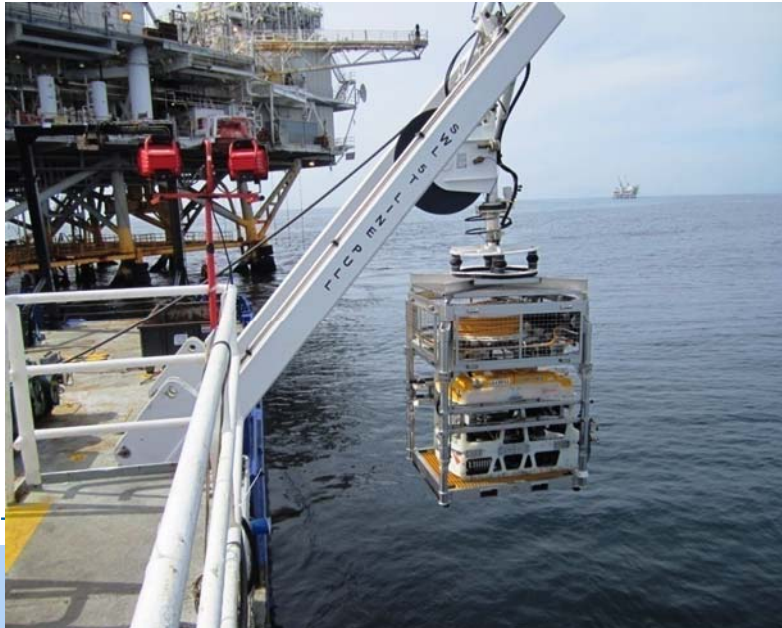
Deployment of "Work Class" ROV for Subsea Inspection
